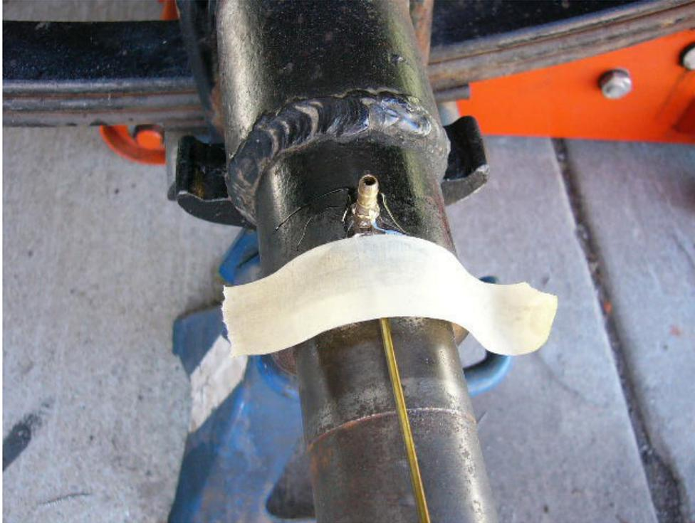
After epoxy is fully cured, remove tape and file away any sharp edges. Some dressing and light sanding will probably be required for proper seal ring fitting. Blow low-pressure compressed air through oil galley to remove any dirt and confirm the passageway is open.
