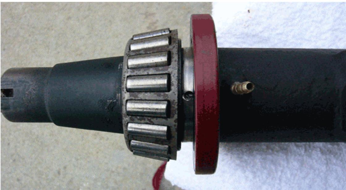
**Image: 8.2** View of oil galley hole drilled in seal ring. Correct location is between inboard bearing and inboard hub seal lip. (Seal shown at running location removed from hub for illustration purposes)
