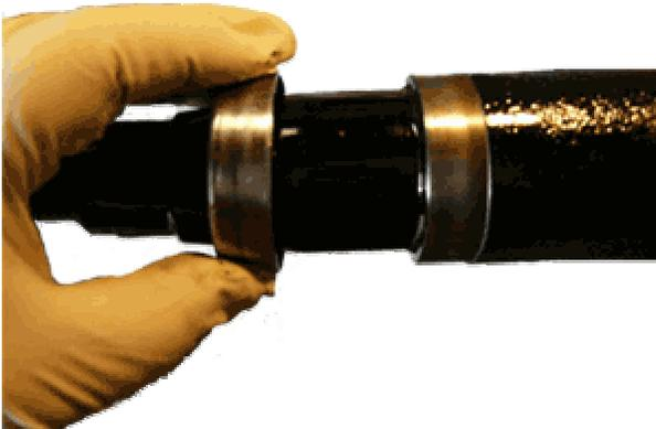
Removing the seal ring
