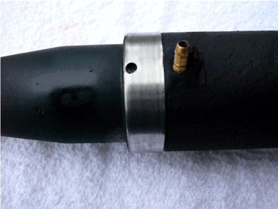
**Image: 8.1** Oil galley hole drilled in seal ring
