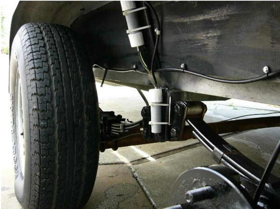
Compy Lub System installed on tandem axle boat trailer.
