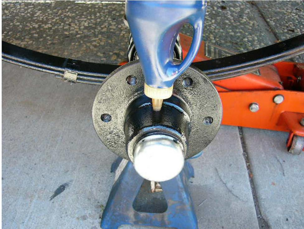
Road Test: Start with short trips (one or two miles) checking oil level periodically. It will take several thermal cycles for trapped air to work out of the system. Add oil as needed to maintain 1/4 to 1/3 cold oil level in reservoir. It will vary with temperature.
